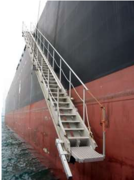
Vessel's gangway deployed for boarding. Bottom platform should be perpendicular to waterline for safe boarding. Adjustments should be made by vessel's crew when necessary.
