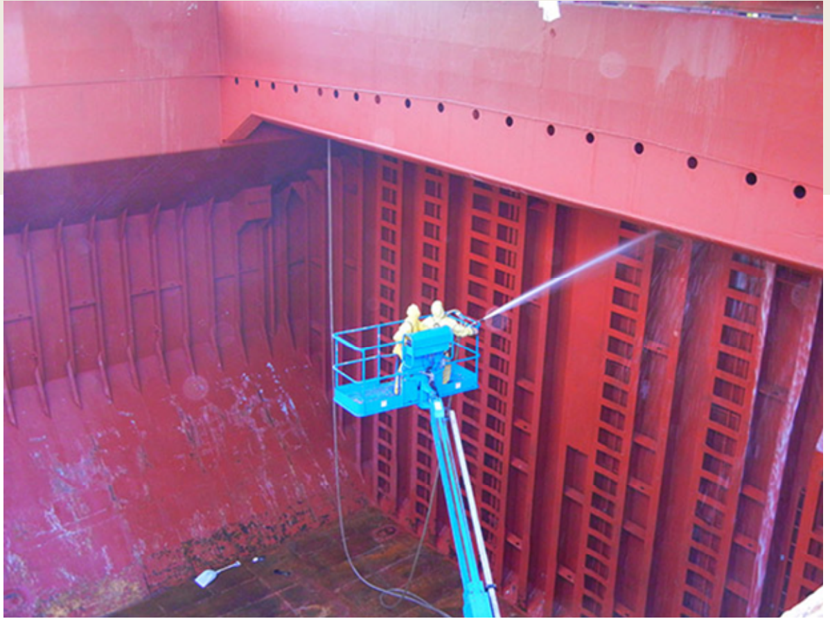
CAPTION: Crew conduct hold cleaning with high-pressure hose and cherry-picker, to access high areas of the cargo hold.
