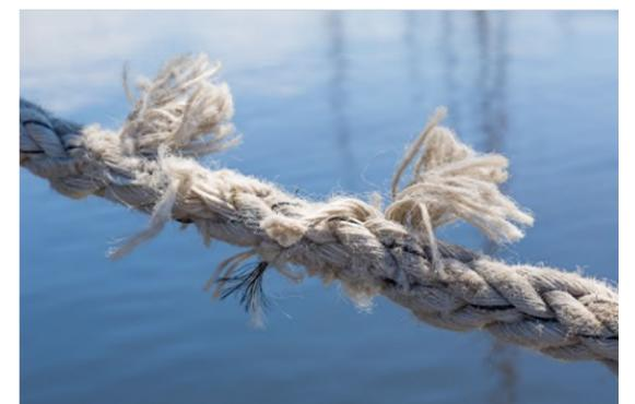
**ABOVE: Mooring lines with frayed or broken strands are much more likely to break under stress. Make note of any such lines and avoid direct proximity for prolonged periods of time.**
