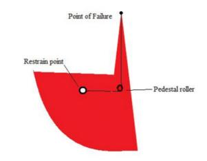
ABOVE: "Snapback points" are areas on deck where a parted line can cause significant injury or death by whipping or 'snapping' back. These areas (indicated in red above) are different for every mooring arrangement, and should be avoided at all times.
