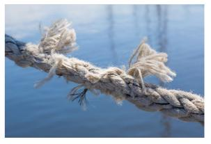
ABOVE: Mooring lines with frayed or broken strands are much more likely to break under stress. Make note of any such lines and avoid direct proximity for prolonged periods of time.
